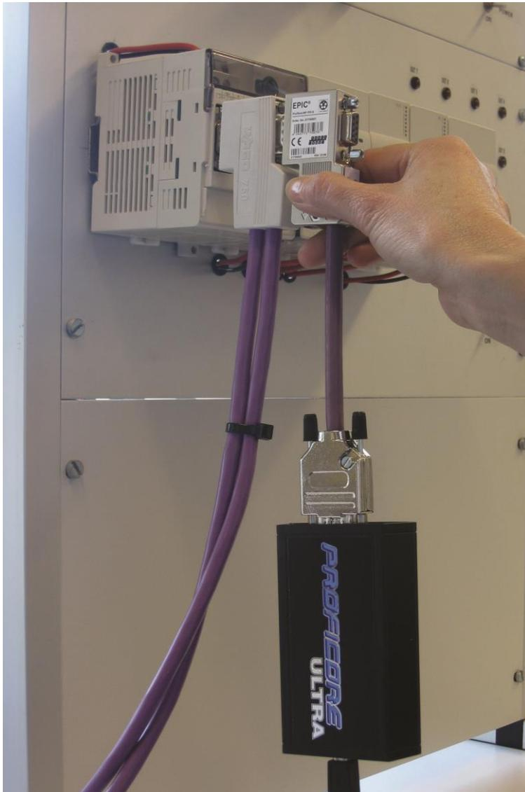
Fig. 10 - Attaching the ProfiCore to a DP installation
