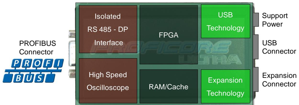
Fig. 2 - Internal structure of the ProfiCore Ultra
