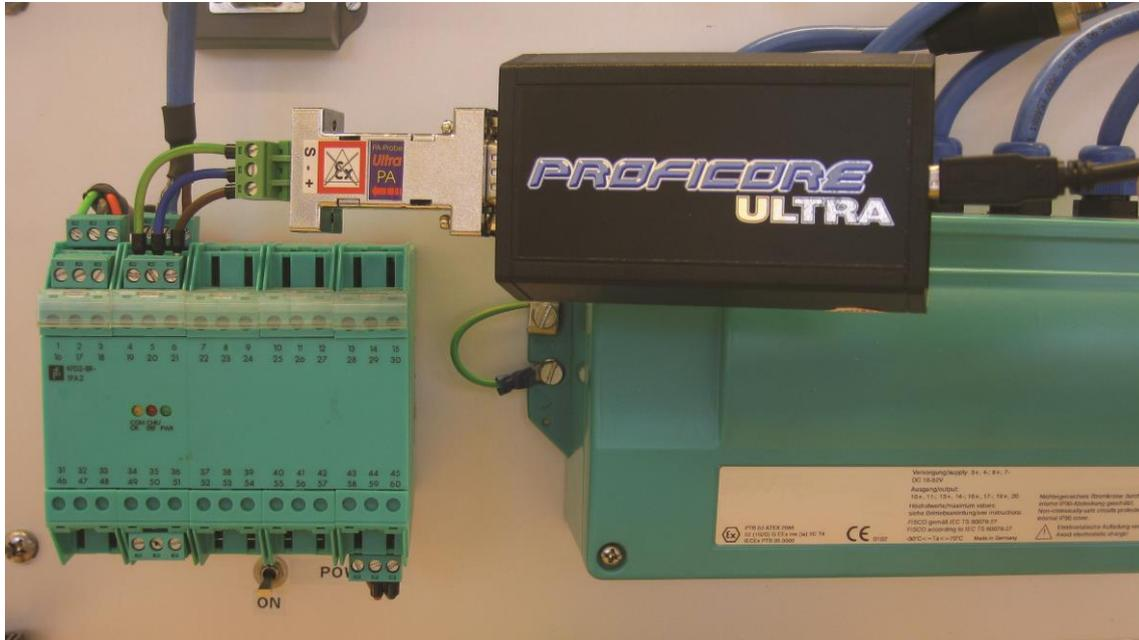
Fig. 12 - Attaching the PA Probe to the installation
